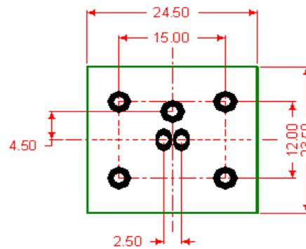
●  $\varnothing 1.50$  PTH HOLE x  $\varnothing 2.00 \times 3.20$  PADS
